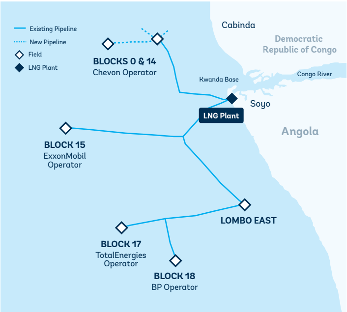
Figure 11 Schematic showing offshore blocks feeding associated gas into ALNG
